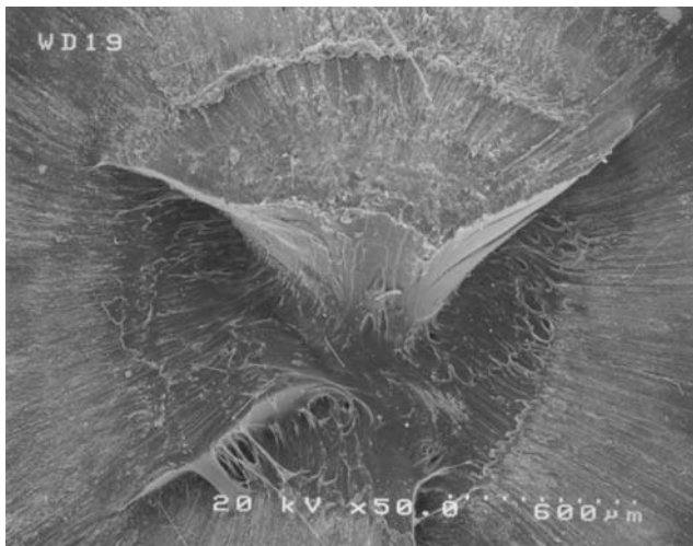
Fig. 3.7 Scanning electron micrograph of healed EMAA-0.3Na film following puncture with a 4.5-mm-diameter projectile [42].
