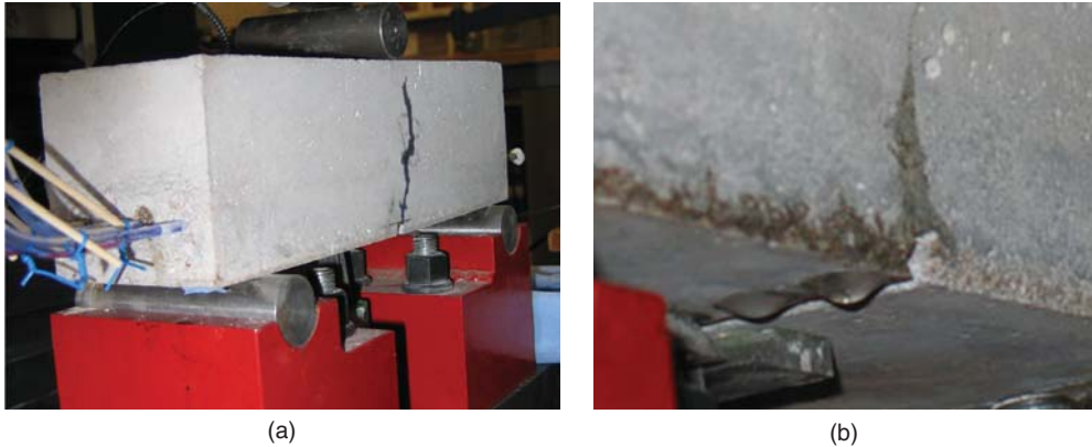
Fig. 5.27 (a) Ink staining during control test and (b) glue seepage during SH test.
