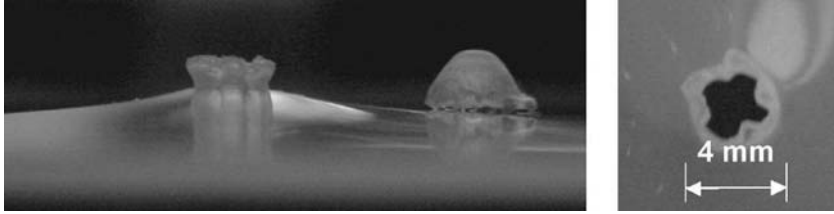
Fig. 3.8 Ballistic puncture damage in LDPE films (reproduced from Kalista et al. [6] www.informaworld.com ).
