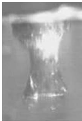
Fig. 3.15 Profile view of partially healed EMAA-0.3Na film tested using impression technique (reproduced from Huber and Hinkley [28]).
